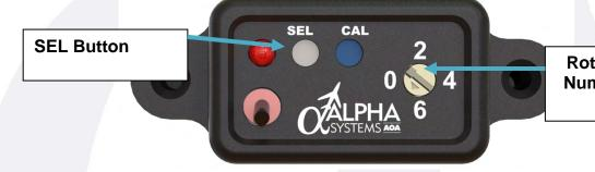
Rotary Switch in Setting Number 1 for Zero Offset Calibration
